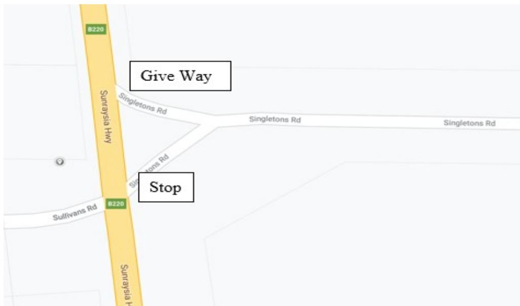
The request details that the safety issue is due to the angle on the Southern leg of the intersection. This justifies the use of the "Stop" sign at this location.
