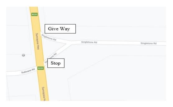
The request details that the safety issue is due to the angle on the Southern leg of the intersection. This justifies the use of the "Stop" sign at this location.
